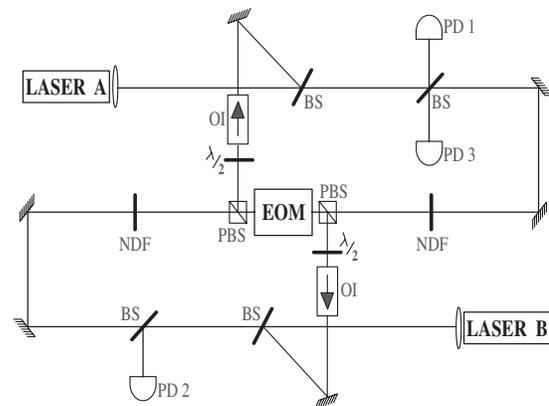
FIG. 2. Schematic of the two mutually coupled lasers. EOM: Electro-optic modulator; BS: beam splitter; PBS: polarizing beam splitter; OI: optical isolator; NDF: neutral density filter; PD: photodetector.
