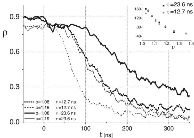
FIG. 3. Experimental results for  $\rho$  as function of  $t$  for  $p = 1.08, 1.19$  and  $\tau = 12.7, 23.6$  ns. Each data point was averaged over 500 measurements. Inset: Data collapse,  $1.7t_d$  ( $t_d$  measured in nanoseconds) versus  $p$  for  $\tau = 12.7$  ns (23.6 ns).
