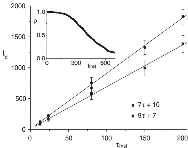
FIG. 1.  $t_d$  as a function of  $\tau$  for  $p = 1.2$ ,  $\kappa = \sigma = 50 \text{ ns}^{-1}$ , and  $C_d = 0.9$  (■) and  $C_d = 0.8$  (●). The lines are a result of a linear fit, and the error bars were obtained from 50 independent calculations for each point. Inset: The average  $\rho$  as a function of time for the same parameters as in the main figure and  $\tau = 50 \text{ ns}$ .
