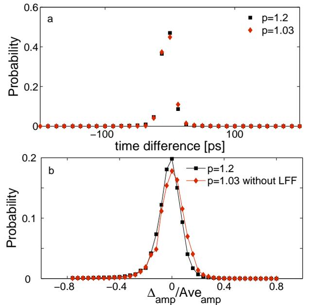
FIG. 6: Two lasers in a zero-lag isochronal phase with a partially transmitting mirror in the schematic of Figure 1. (a) The histogram of the mismatch in the timing of spikes of the two lasers, and (b) the relative ratio between the maximum of the intensity of temporally correlated spikes of the two lasers.
