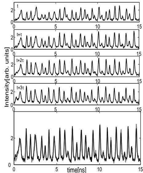
FIG. 2: A trace of 15 ns duration of the intensity of one laser followed by plots of the same laser intensity after a time  $\tau$ ,  $2\tau$  and  $3\tau$  with  $\tau = 23.55$  ns. The laser was operating with  $p = 1.03$  and with a reflected power of a few % of the laser output intensity. In the bottom panel the intensity trace at time  $t + \tau$  and at time  $t + 2\tau$  are superimposed, demonstrating the slowly decaying periodicity of the spiking pattern.
