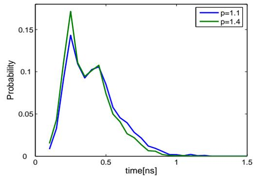
FIG. 5: Two lasers in a face-to-face configuration corresponding to a fully transparent mirror in the schematic of Figure 1. The first laser operates with  $p = 1.1$  and the second laser with  $p = 1.4$  and the coupling strength is a few % of the laser intensities. The probability for the time intervals between spikes is presented for each one of the lasers. The two maxima correspond closely to the refractoriness of the solitary lasers operating with  $p = 1.1$  and  $1.4$  (see Figure 3).
