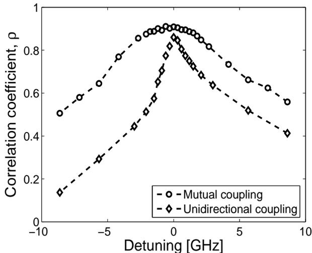
Figure 6: Correlation coefficient as a function of detuning of laser  $A$ 's optical field's frequency in respect to laser  $B$ , for mutual (open circles) and unidirectional (open diamonds) coupling. Feedback strengths are  $\sigma_0$  and  $\kappa_0$ .
