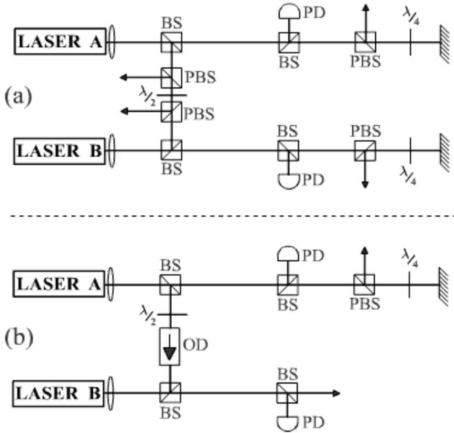
Figure 1: A schematic figure of the two coupled lasers for the mutual (a) and unidirectional (b) cases. BS - Beam Splitter; PBS - Polarizing Beam Splitter; OD - Optical Isolator; PD - Photodetector
