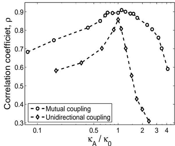
Figure 5: Correlation coefficient for different values of  $\kappa_A$ , laser A's self feedback rate. Coupling strength is  $\sigma_0$ .  $\kappa_b = \kappa_0$  and  $\kappa_b = 0$  in the mutual (open circles) and unidirectional (open diamonds) coupling, respectively.
