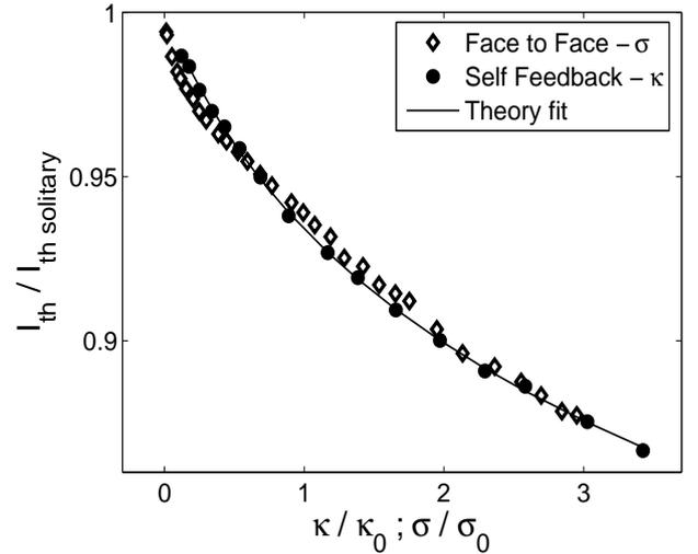
Figure 2: Measurements of the relation between the amount of feedback a laser is subjected to and the effect of reduction in its threshold current.  $\sigma_0$  and  $\kappa_0$  are the equivalent for a 6.6% reduction in  $I_{th}^{sol}$ . Theoretical fit is according to eq.1 (see text).
