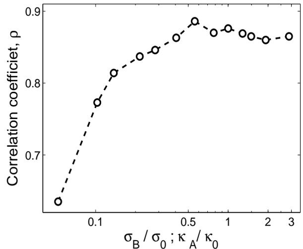
Figure 4: Correlation coefficient as a function of  $\kappa_A$  and  $\sigma_B$ , the self feedback of laser A and the coupling to laser B, respectively, for unidirectional coupling.  $\kappa_A = \sigma_B$  at all time.
