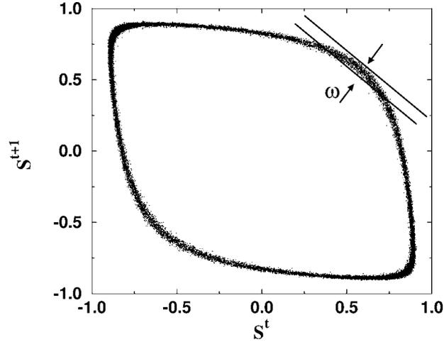
Figure 8. A broadened attractor generated by a perceptron-SGen,  $N = 50$ ,  $K = 17$ ,  $\beta = 1/17$ ,  $\phi = 0.123$  with a uniformly distributed noise of amplitude  $\pm 0.1$  added, equation (32).  $\langle \omega \rangle$  denotes the width perpendicular to the attractor.
