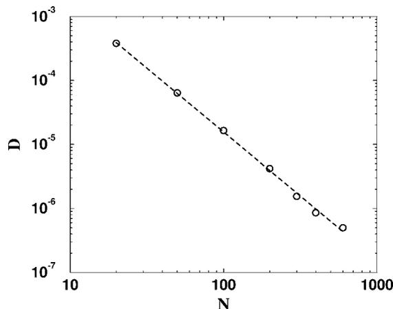
Figure 9. Diffusion coefficient obtained by simulating the system for several system sizes (over a decade). The linear regression (dashed line) is  $D = 0.154/N^a$  with  $a = 2 \pm 0.036$ .
