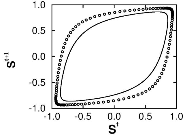
Figure 4. Two-dimensional embedding of a sequence generated by a perceptron whose weights follow equations (15), (18). The parameters for the periodic sequence are  $N = 128$ ,  $K = 17$ ,  $b = 0.3$ ,  $\beta = 1/40$  and for the quasi-periodic  $K = 17$ ,  $\phi = 0.123$ ,  $\beta = 1/45$ , respectively.
